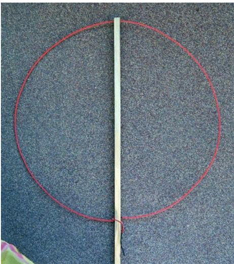
**Fig.3.3** Single turn loop with 6mm<sup>2</sup> PVC insulated Cu wire
