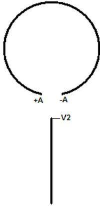
**Fig.3.2** Connect Loop at +A, -A terminals. J1a=ON, J1b=OFF. Connect short counterpoise at V2 terminal.
