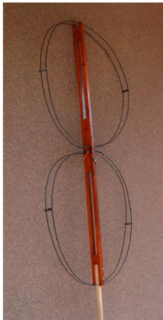
**Fig.3.7** This is the basic loop/dipole design
